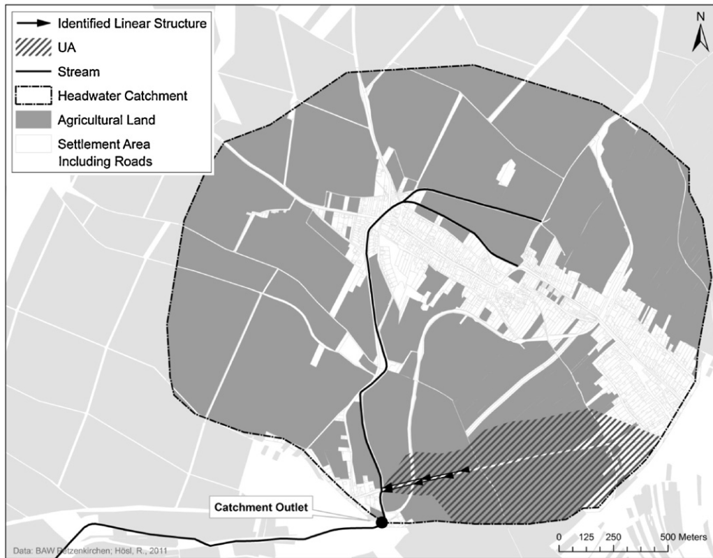
Fig. 2. Headwater catchment in the Weinviertel region. Identified linear structures and unprotected areas (UA) by using the Advanced calculation method and DEM 1 m.
