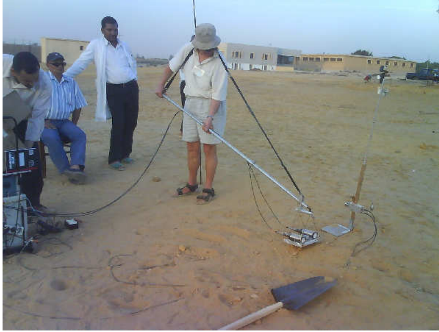
Fig. 2: The hand-held HYDAD-D sensor in action at the Inshas Centre, Egypt.
