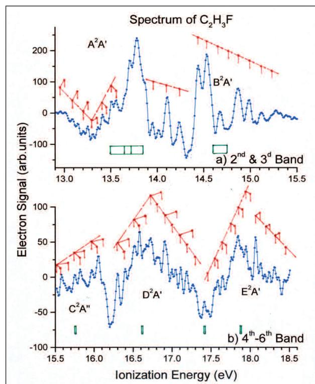
▲ Electron signal resulting from photoionization to electronic excited states of  $C_2H_3F^+$ . The vibrational structure (red markers) has been amplified by a continuum subtraction procedure. The green areas locate the fragment appearance energies.
