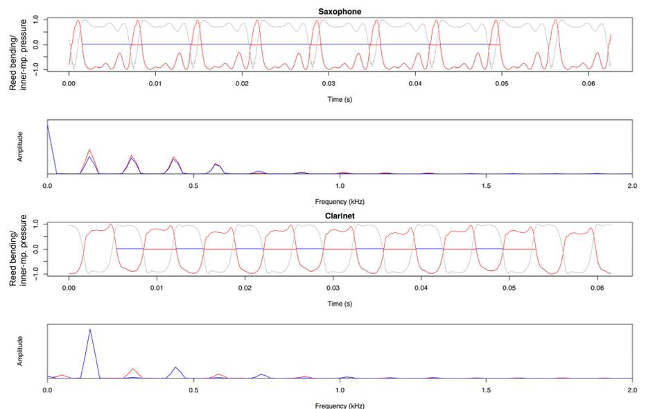
Waveforms (top) and Spectrum (below) for a the tone D3, played on saxophone and clarinet. Reed bending (red) and inner-mouthpiece pressure (grey/blue).
