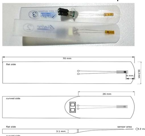
Left: Mouthpiece with piezo-resistive pressure transducer. Right: Synthetic single reed with strain gauge sensor.
