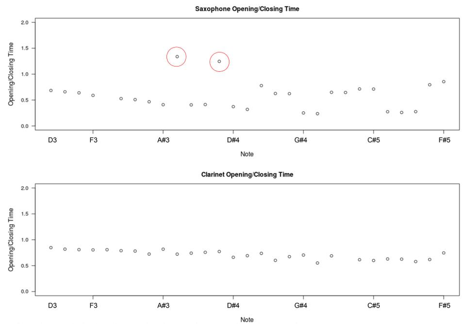
Opening and closing time ratio of saxophone and clarinet reeds.
