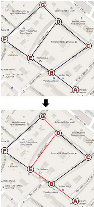
Figure 1: An example of a graph superimposed on a geographical map with nodes A , B , C , D , E , and F . Edges show the direct paths between the locations. The edge weight corresponds to the distance (measured in meters) between the locations. The red path shows the shortest route between A and G with respect to the total distance covered. Map data ©2016 Google
