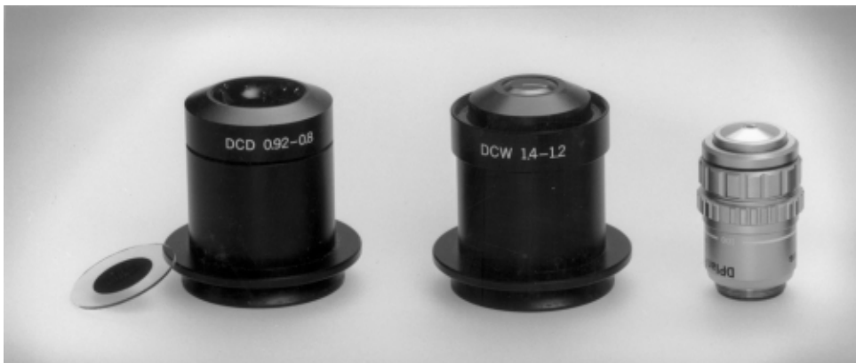
Figure 3 Equipment for darkfield microscopy. From the left: a patchstop, a dry darkfield condenser, an immersion darkfield condenser, and an oil-immersion objective with iris diaphragm.
