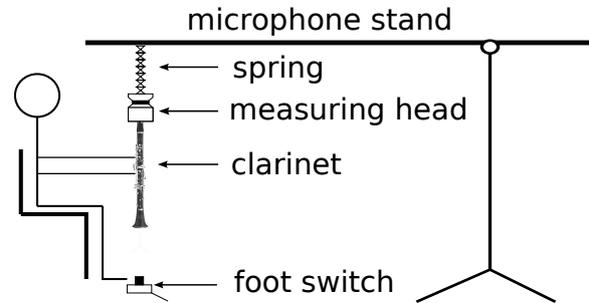
Figure 5: Measuring method using a microphone stand with a spring to reduce the weight of the measuring head and the instrument for the player.
