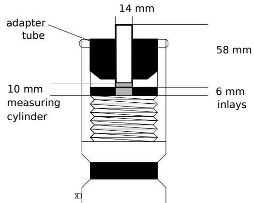
Figure 6: Cross section of the BIAS measuring head with new customized adapter tube, replacing the Eb-clarinet mouthpiece.
