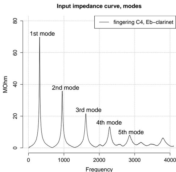
Figure 1: An input impedance curve can be subdivided into several modes.
