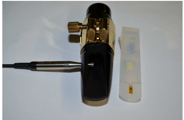
Figure 1. Vandoren AL3 mouthpiece with microphone attached (left); Synthetic saxophone reed with 2mm strain gauge sensor (right)
