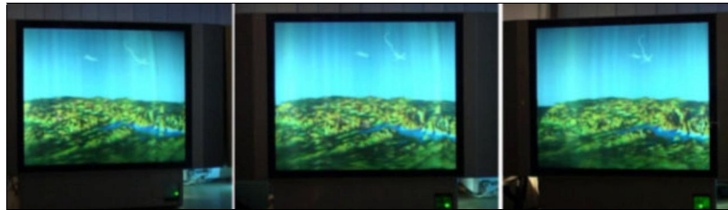
Figure 5: Visualization of a real air traffic situation in 3D by means of a quasi-holographic display and the digital map of Hungary (“HoloVizio”-display from Holografika) ( www.holografika.com )
