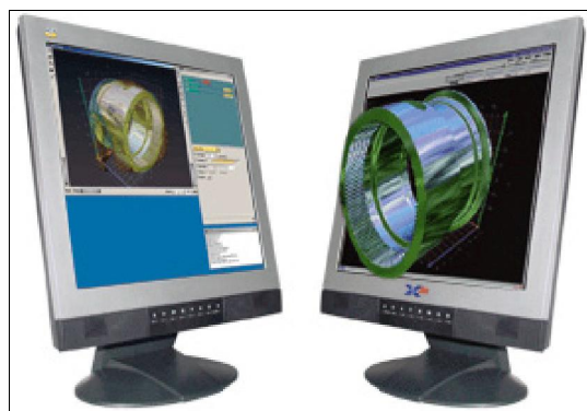
Figure 4: An interactive autostereoscopic application, based on the “OpenGL Enhancer”; left side: conventional display, including the GUI; right side: autostereoscopic visualization via multi-view parallax-barrier method ( www.x3dworld.de or www.opticalitycorporation.com )
