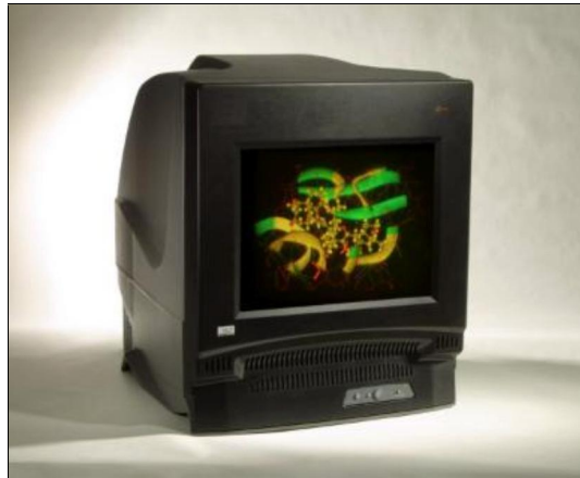
Figure 2: “Depth Cube Z1024 3D” – a volumetric multi-directional, multi-level display made up of twenty stacked LCD-layers ( www.lightspacetechnology.com )
