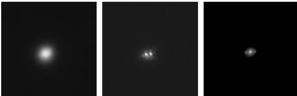
Figure 1. Left: A long (125 sec) exposure of a star. Middle: The same star in an image exposed for only 0.5 sec. Right: An image of the star obtained with the Shift-And-Add method, using about 125 input images. The field-of-view of the images is 6.4'' .
