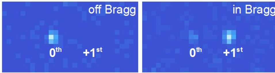
Figure 2: Left: 2D-detector matrix at off-Bragg position. All the intensity is transmitted to the 0 th diffraction-order spot. Right: 2D-detector matrix at the Bragg-angle. Here, almost all the intensity is diffracted to the +1 st diffraction-order spot. The grating acts as a mirror with reflectivity 0.9 .
