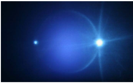
FIG. 1. (Color online) Far-field readout diffraction pattern of a H-PDLC fabricated from a 50/50 mixture of TL203 and PN393. The right spot is the transmitted beam and the left spot is the first-order diffracted beam. Bright rings with different diameters are related to holographic scattering. Recording and readout wavelength is 351 nm.
